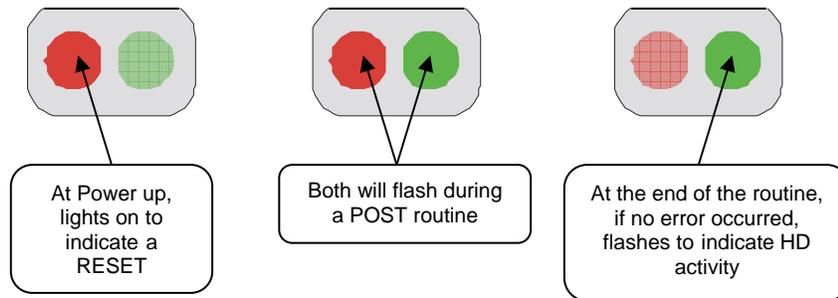
At the beginning of each POST routine, the debug LED lights YELLOW (both LEDs light on). If the BIOS detects an error condition, it halts POST after issuing an error post debug code and the LED will light RED indicating an error.
