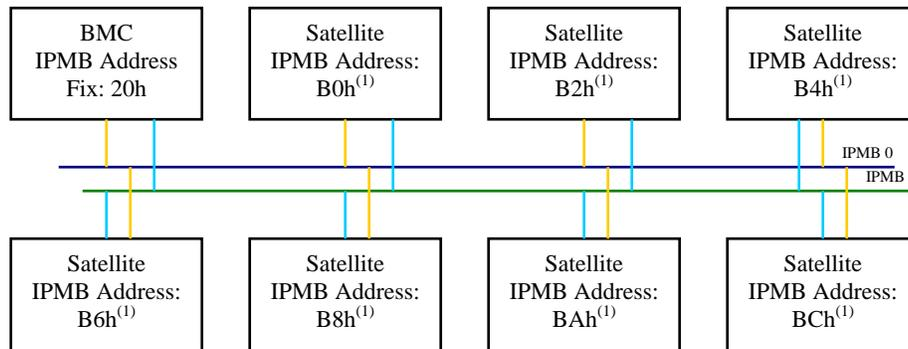
( 1 ) IPMB address for satellite is determined via the location of the slot in the chassis
