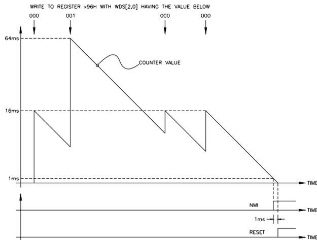
The programmable watchdog can be viewed as a decremting counter that is initialized by a write to register x96h. The processor must initialize the counter to prevent it from reaching count 0 (timeout).
